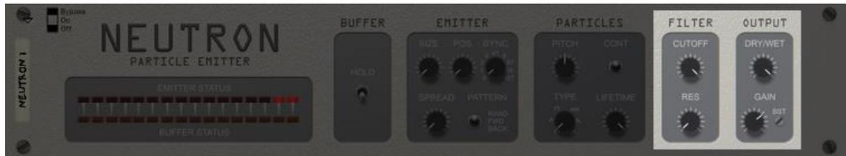
The filter is a resonant low-pass filter that you can use to remove high frequencies from the sound extracted by the particles. The filter has two properties: *cutoff frequency* and *resonance*. A high cutoff value will preserve the audio as-is, while a low cutoff value will remove higher frequencies from the audio. The resonance property controls the resonance of the filter; at high values the filter becomes self-resonating.
