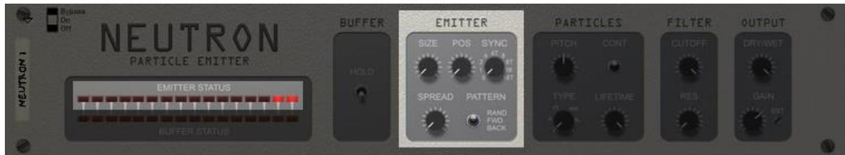
The particle emitter has variable *size* and *position*. These two properties determine where in the sound buffer particles will be created. When the emitter is at its widest size it will create particles that extract bits of sound from across the entire sound buffer, which means that the sound you hear will be pieced together from the last eight seconds of input. When the emitter is at its smallest size, the sound you hear will be extracted from a small piece of the buffer.
