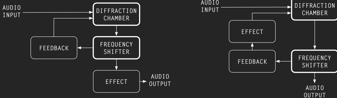
In the leftmost image above, the effect unit has been placed after the main feedback loop. This allows the effect unit to process the full output of the feedback loop.
