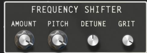
The AMOUNT knob controls how much of the input to the frequency shifter that should be processed. It is essentially a "dry/wet" knob for the frequency shifter.
