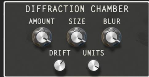
The AMOUNT knob controls how much of the input that should be processed. It is essentially a "dry/wet" knob for the diffraction chamber.
